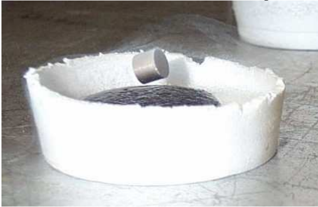
Figure 2-6 – A combination of the Meissner effect (Type I) and flux pinning (Type II) gives us stable levitation
