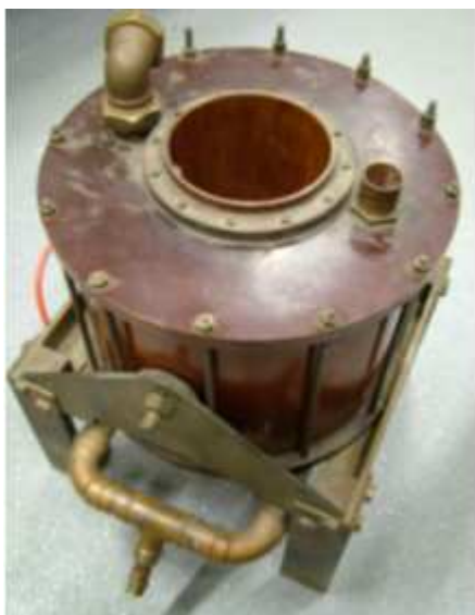
Figure 1-4 – A liquid nitrogen cooled solenoid. Most of the space is occupied by the cooling coils!
