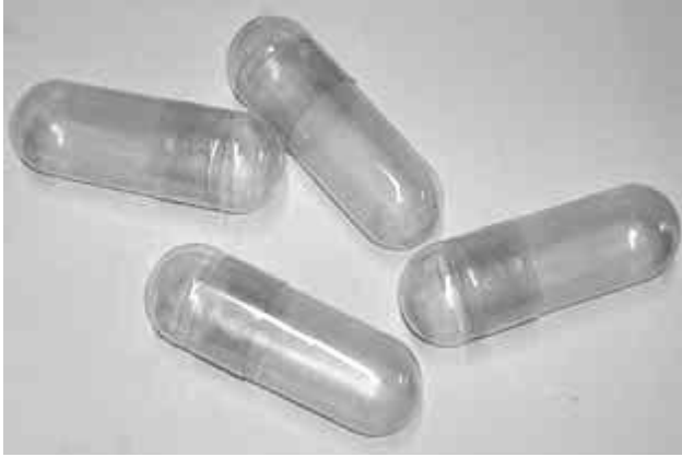
Figure 7-5 – Gelatine pill capsules used for mounting powder in the SQUID
